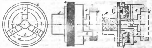
FIG. 39.—Scroll Chuck, ungeared.
